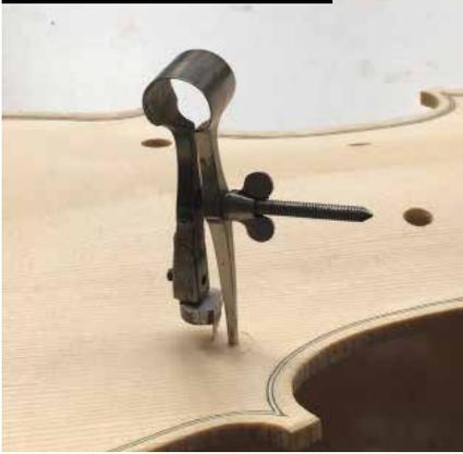
I can check and decide to follow the original layout, or if I should divert from it by extending the distance between the lower eyes. Once I'm fully satisfied, I drill the lower eyes.
