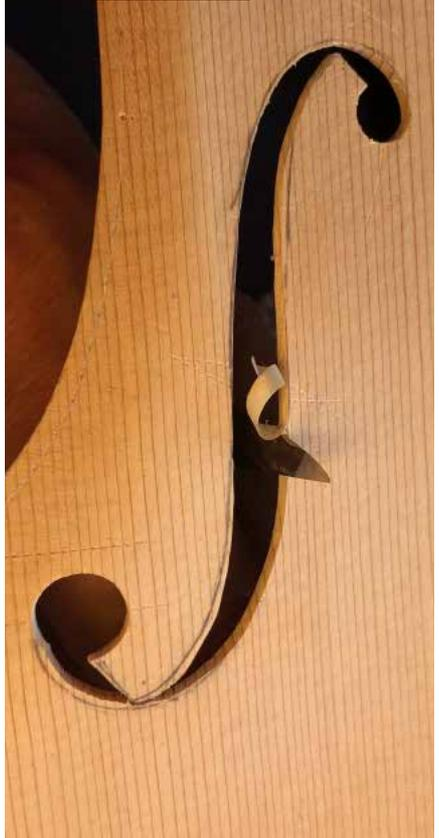
**FIGURE 6** The finished f-holes seen from the inside
